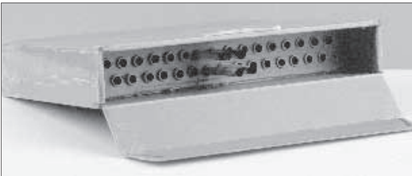
Figure 17. Paraffin-coated cardboard box with cardboard tubes and inserted paper straws.
